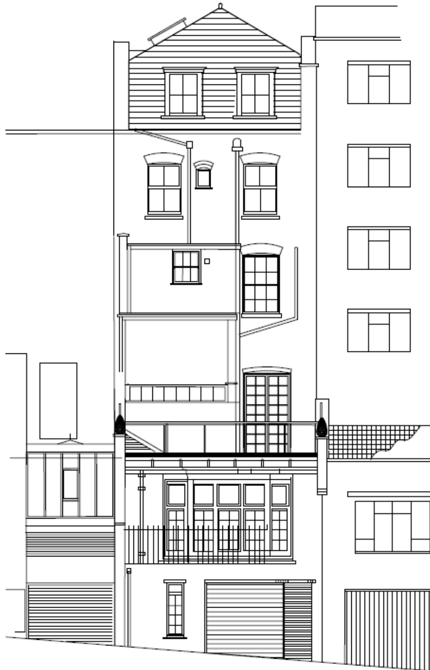
Rear Elevation 1:50 Proposed roof terrace
